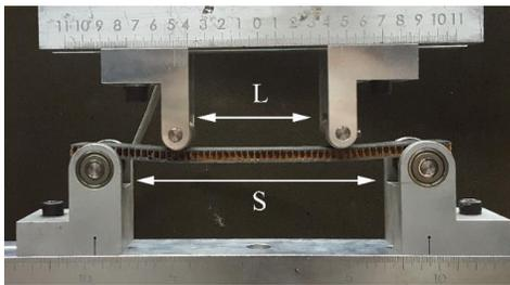
Fig. 2. Setup used to perform four-point bending tests.  $S$  represents the outer load span and  $L$  the inner load line.
