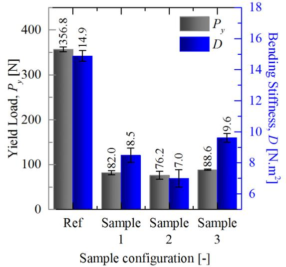
Fig. 5. Bending stiffness of all samples obtained from four-point bending tests.
