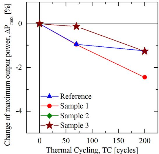
Fig. 3. Results from TC from 2-cells mini-module. Electrical properties are analyzed after 70 and 200 cycles. *Sample 2* failed after few cycles so its electrical performance could not be measured.
