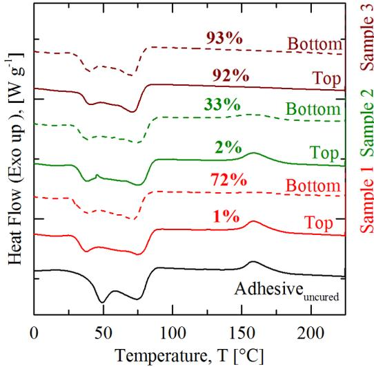
Fig. 4. DSC measurements obtained for an uncured adhesive (no processing), *Sample 1, 2 and 3* (top and bottoms refers to close, respectively far from the heating plate).
