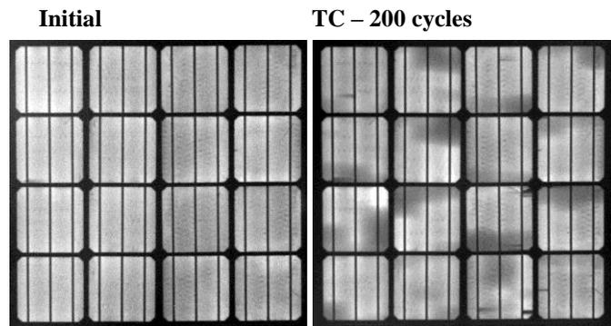
Fig. 7. EL images of one module tested under TC before and after 200 cycles.
