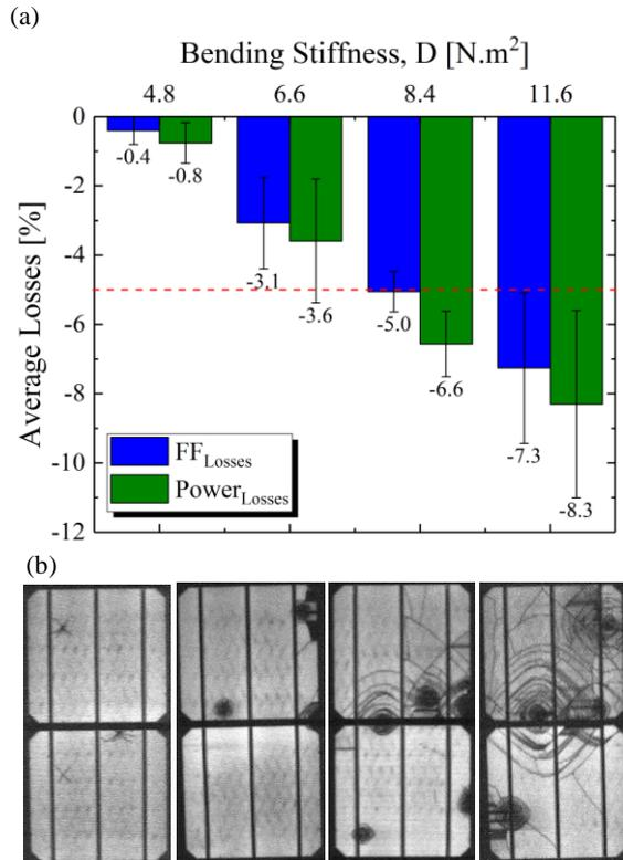
**Figure 3:** (a) Power and fill factor losses for our mini-modules after the hail test and (b) corresponding EL images. The test devices were manufactured using backsheets with different bending stiffness's.
