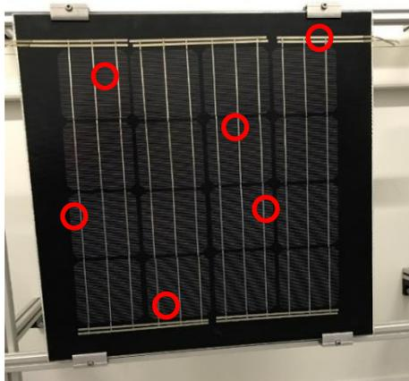
**Figure 5:** Medium-area module with indication of the impact spots used for the hail test.
