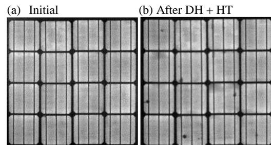
**Figure 6:** EL images of medium area modules composed of a stiff composite backsheet and a thin polymer frontsheet.
