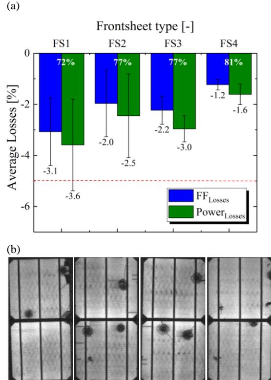
**Figure 4:** (a) Power and fill factor losses after the hail test for our 2-cells mini-modules with different frontsheet, and (b) the corresponding EL images after the ice-balls impact.
