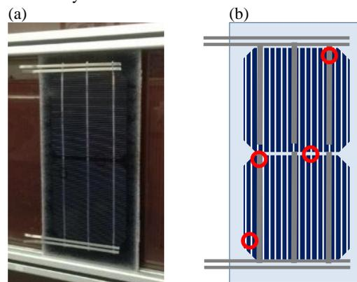
**Figure 2:** Hail test setup (a) example of fixation system used on two-cell mini-module during the hail test and (b) impact spots for the hail test.
